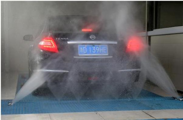
Leisuwash S90 car wash machine is equipped with a unique chassis and fan-shaped flushing wheel function. The 90kg high-pressure flushing can effectively clean the chassis, the body and the sediment of the hub.
